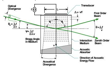
A plot of incident and diffracted angles illustrates isotropic phase matching (Bragg angle) is always sensitive to the incident angle regardless of wavelength ( $\lambda_{\circ}$ ), frequency (f) or velocity (v).
