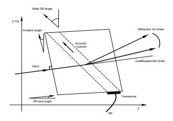
Case 2: Off-axis modulator/deflector, orientation B
